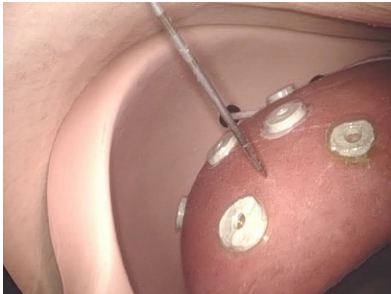
Figure 9: Control view: an endoscopic camera is inserted inside the phantom to check the targeting accuracy.
