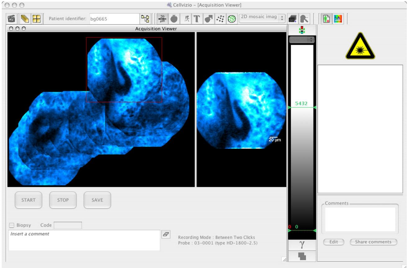
Figure 3: The graphical user interface of the live mosaicing. The clinician can see on the same screen, the regular acquisition view on the right and the simple mosaic, stitched on-the-fly, on the left. Courtesy of PD. Dr. A. Meining, Klinikum rechts der Isar, Munich.
