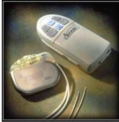
Figure 1.2: The Medtronic® Kinetra neurostimulator (bottom-left) and its Access Therapy Controller (top-right), allowing its control by a physician. The implanted stimulator is about the size of a watch. Image courtesy of Medtronic, Inc.
