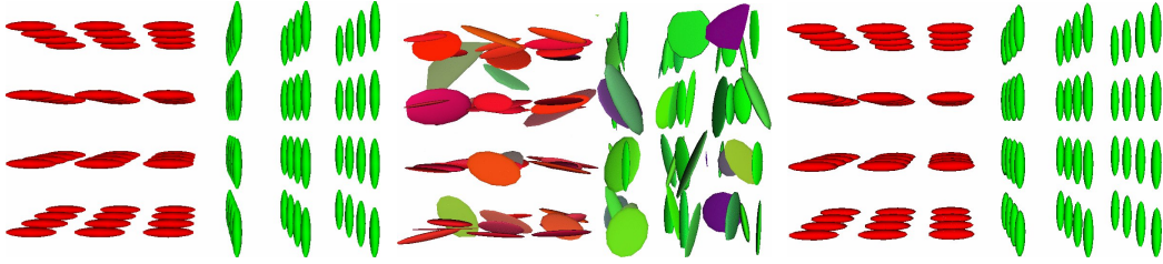
Figure 4.10: Left: 3D synthetic tensor field with a clear discontinuity. Middle: The field has been corrupted by a Gaussian noise (in the Riemannian sense). Right: result of the regularization after 30 iterations (time step \varepsilon = 0.01 , \kappa = 0.05 ).
