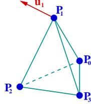
Figure 1:  $P_1$  finite element
