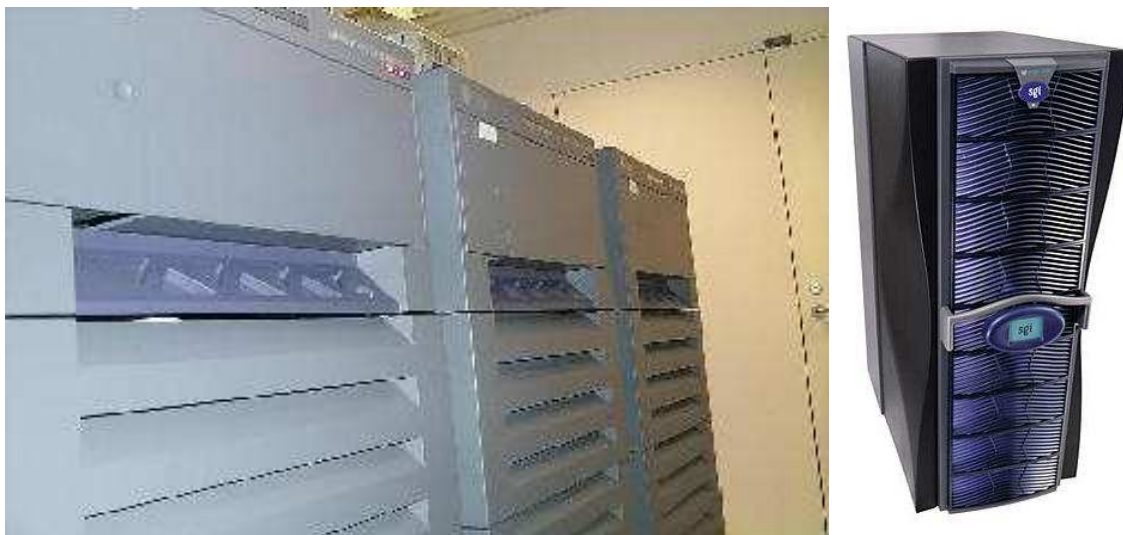
FIG. 7.2 – Left: Wildfire Cluster with scalable memory, architecture built on SUN E5k and E6k chassis, 36 250MHz UltraSPARC-II CPUs and 9GB RAM (source: (Kikinis, 2000a)); Right: SGI Origin 3400, architecture built on 32-processor shared-memory system and 64GB RAM under IRIX 6.5 (source: http://www.sgi.fr/servers/ ).
