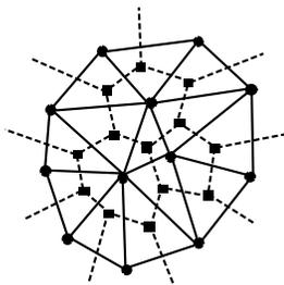
Figure 1: A 2-simplex mesh and its dual triangulation.
