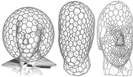
Figure 4: **Left** The initial mesh is a sphere with 720 nodes; **Center** the mesh is fit on the surface. The mesh grossly approximates the surface because it is smoothed over a large extent and because the mesh is not adapted; **Right** The mesh is now iteratively adapted and refined. We chose a small value of  $\gamma_i = 0.06$  and a medium threshold for controlling the refinement;
