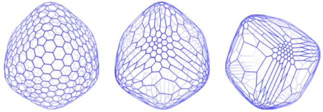
Figure 2: **Left** the mesh fit on the isosurface. The metric parameters are everywhere equal to  $\frac{1}{3}$ ; **Center** The adaptive mesh with a value of  $\gamma_i = 0.15$ ; **Right** The adaptive mesh with a value of  $\gamma_i = 0.20$ .
