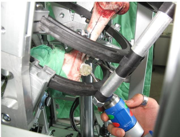
**Fig. 3** Digitising. The markers used, can be easily digitised, a sample reference frame cube is shown, mounted on a porcine model within the experimental set up
