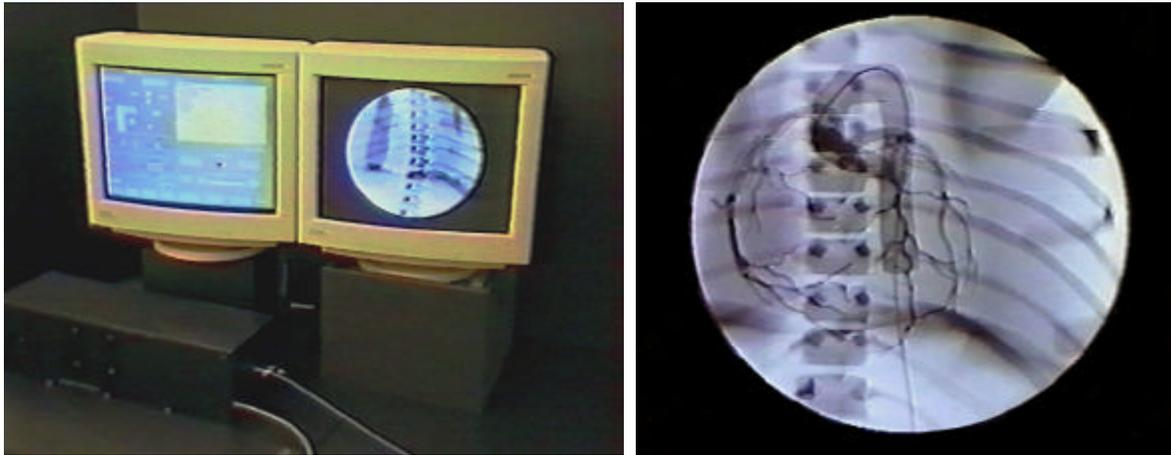
Figure 5 – (Left) A picture of the ICTS prototype with the haptic device in the foreground. (Right) a screenshot of the simulated fluoroscope showing the catheter and contrast moving into the aorta and coronary arteries.
