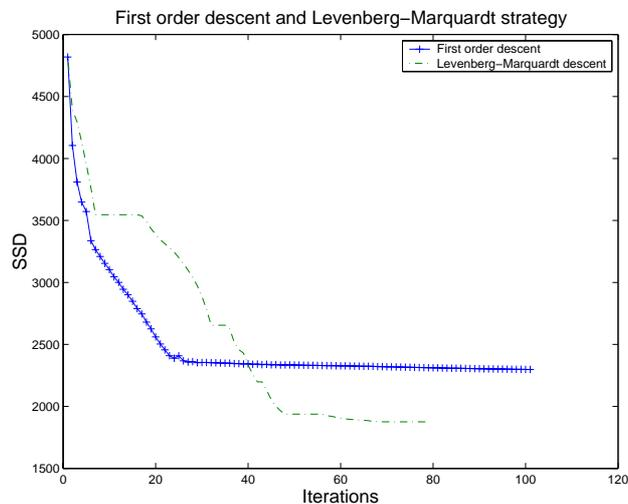
Figure 9: **SSD criterion evolution for a polyrigid registration with a Levenberg-Marquardt (LM) versus a simple first-order optimization scheme.** This shows that using a second-order descent has greatly enhanced the final results quantitatively, and also qualitatively as is shown in the next figures.
