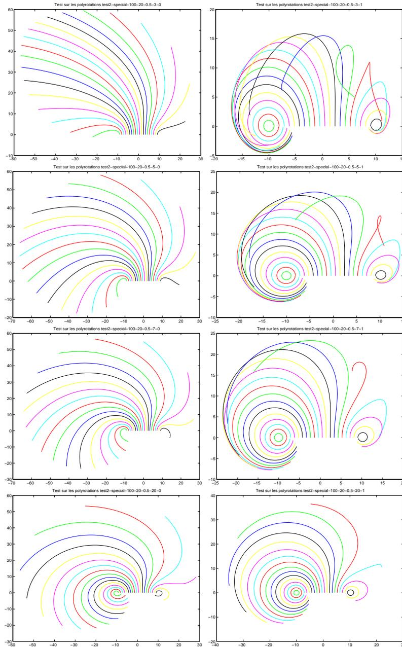
Figure 2: **First scheme (on the left) versus second scheme (on the right).** From top to bottom: discretization levels of 3, 5, 7 and 20. As in figure 1, various trajectories are displayed, these trajectories being obtained when the two opposite rotations see their angle increase progressively between 0 and  $2\pi$ . Here, the rotation on the left has a larger relative weight than that on the right, which lessens the influence of the latter.
