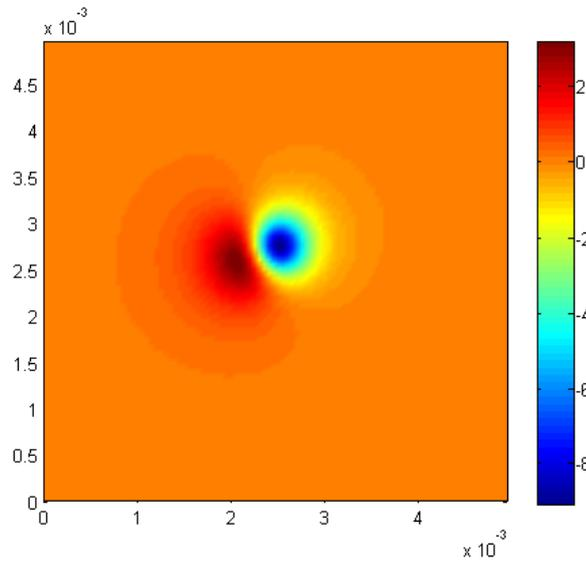
Figure 1: The normal component of the magnetic field of the Lonar Spherule example
