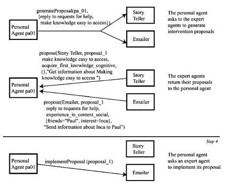
Fig. 5. An example of instantiation of the intervention selection protocol.
