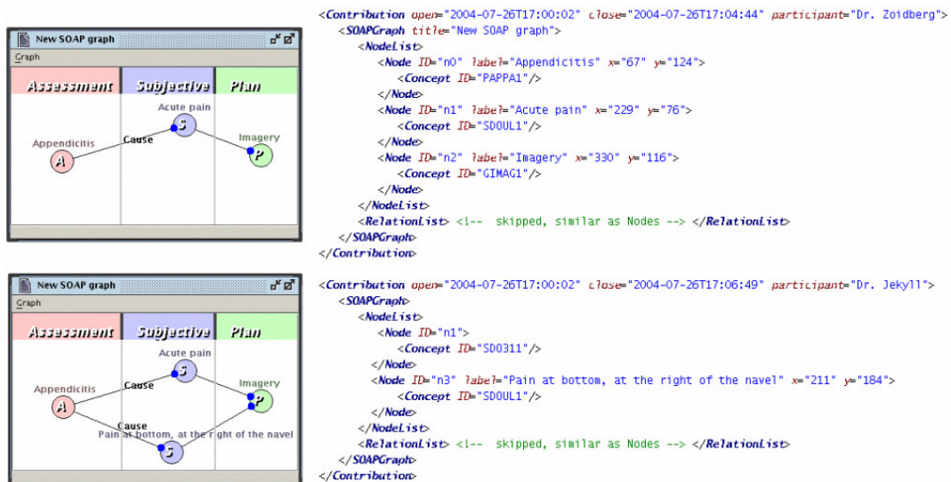
Fig. 6. XML format for storing cases using delta function
